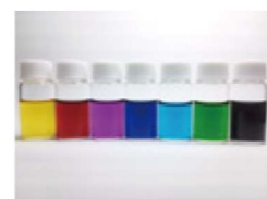
Optical images of the colloidal solutions of silver nanoplates with different sizes (courtesy of Dai Nippon Toryo Co., Ltd.)
